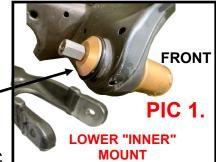
G. Clean hole and insert the new KMAC MOUNT elastomer bushes. Now lubricate the steel inner bushes (only) with silicone grease supplied and insert.
