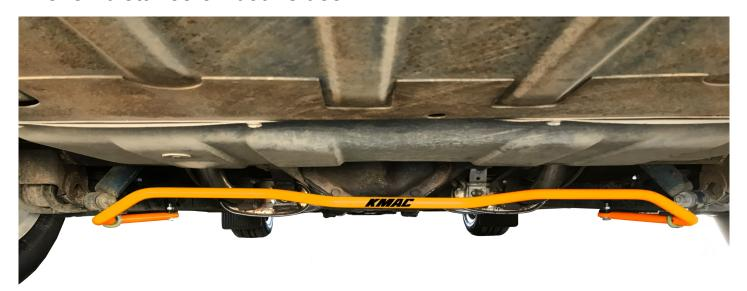
C. Connect each plate to trail arm 'U' channel by centre punching up through remaining hole in each plate. Drill 3/8" hole and insert long bolt supplied with the large flat washer and self lock nut on top. Check all bolts are tight / secure.
