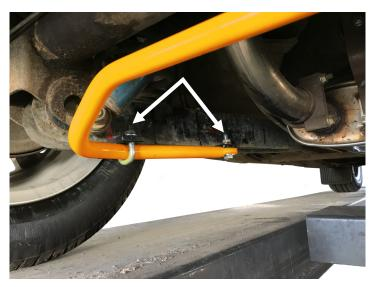
B. Position sway bar as in Pic '2'. With mount plates under each trail arm. Move bar forward as much as possible making sure even distance on both sides.
